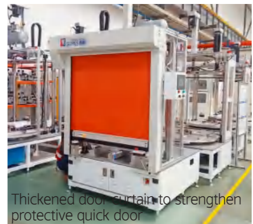
Protective quick door in arc-proof welding room
