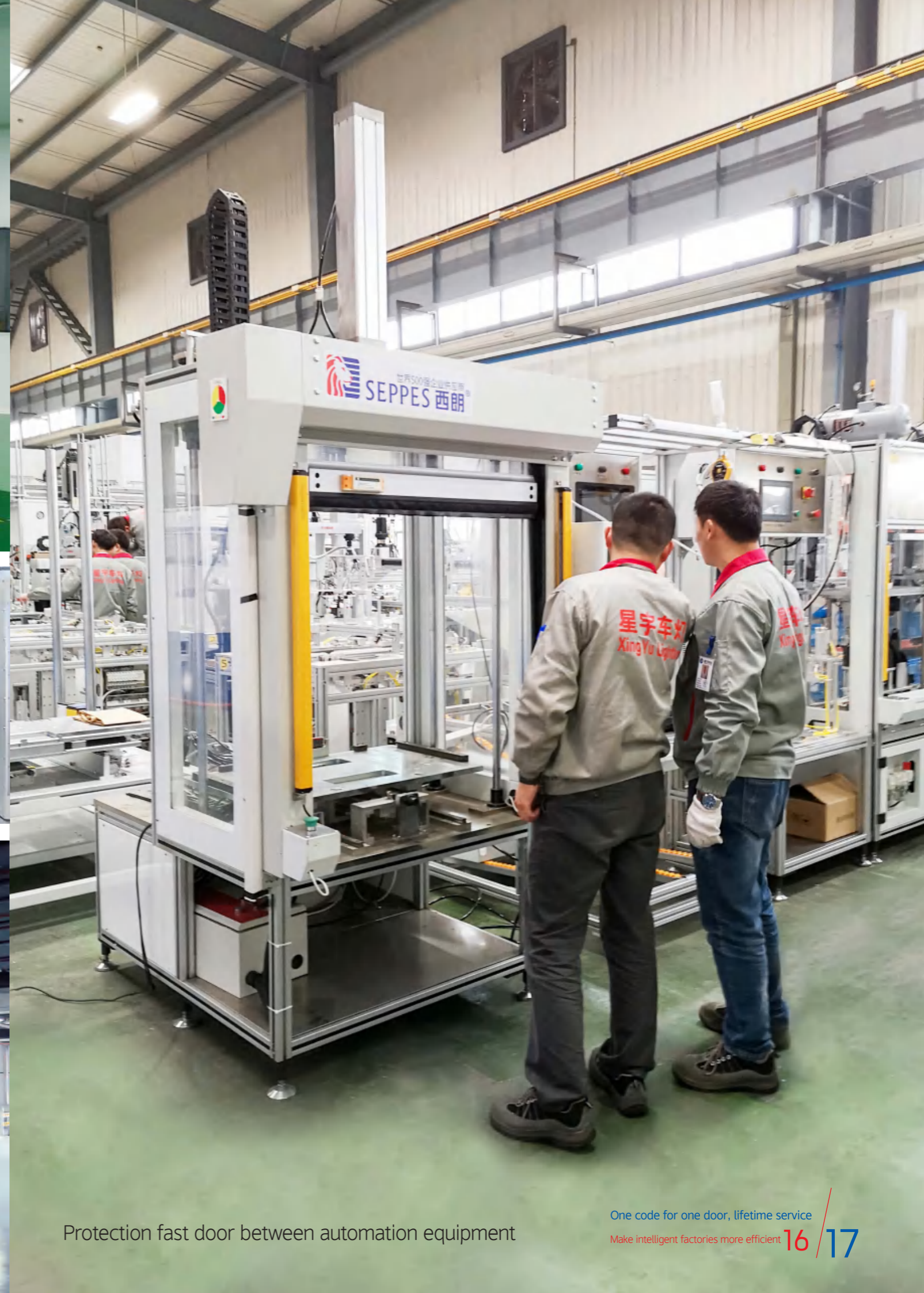
The fast door of the conveyor belt delivery port of the intelligent three-dimensional library (Yangtze River Pharmaceutical Group Factory)
